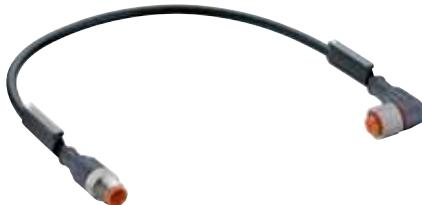
Actuator/sensor cordset, double-ended, M12, 3-, 4-, 5-, and 8-poles, male straight to female 90° connector with self-locking thread and molded cable, IEC color code.
