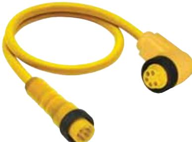
Mini, 7/8" double-ended cordsets, male straight to female 90°, 3- and 6-poles with molded cable, Automotive color code.
