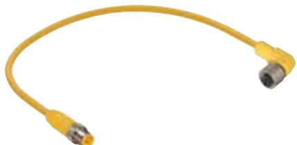
Actuator/sensor cordset, double-ended, M12, 3-, 4-, and 5-poles, male straight to female 90° connector with self-locking thread and molded TPE, PUR, or PVC cable, IEC color code.
