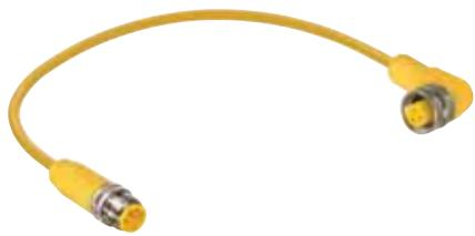
1/2"-20 actuator/sensor-cordsets, single ended, 3-poles, male to female 90° connector, dual keyway, 18 gauge, US color code.
