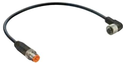
Actuator/sensor cordset, double-ended, M12, 8-poles, male straight to female 90° connector with self-locking thread and molded PVC black cable, IEC color code.
