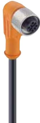
Actuator/sensor cordset, single-ended, M12, 4-, 5-, and 8-poles, female 90 °connector, internal threads with threaded joint and molded cable, shielding connecting to knurled nut.
