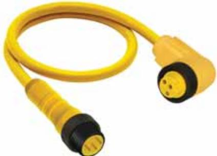
Mini, 7/8" double-ended cordsets, male straight with external threads to female 90° connector, 3-poles with molded cable, IEC color code.
